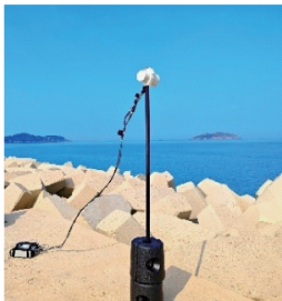
(b) 地面部署 Overhauser 磁力仪 (b) Ground deployment of the Overhauser magnetometer
