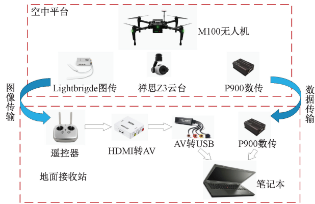
Fig. 8 Track experiment platform architecture
