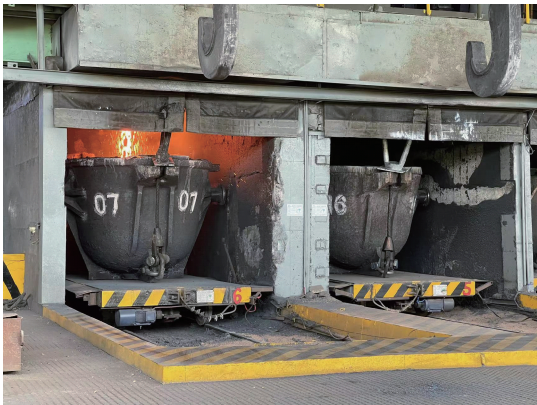
图 14 贫化区产出低镍钼过程 Fig. 14 Process of producing low nickel matte in depleted area
