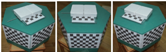
(b) 测量b组角点的三视角图像 (b) The three view-angle images for measuring the corners in group b
