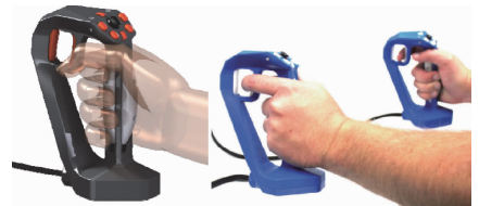
图 9 基于剪切力的力触觉再现装置 Fig. 9 Haptic rendering device based on shearing force
