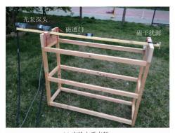
(a) 实验木质支架 (a) Wooden shelf with OPMs,fluxgates and interference sources
