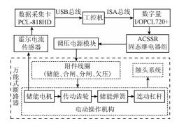
图 1 基于储能电流的操作机构故障检测系统 Fig. 1 Fault detection system of operating mechanism based on storage current
