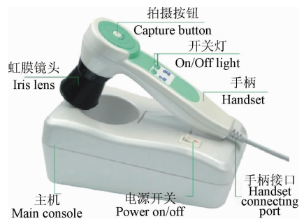
(a) 采集图像的虹膜仪 (a) Capturing image instrument
