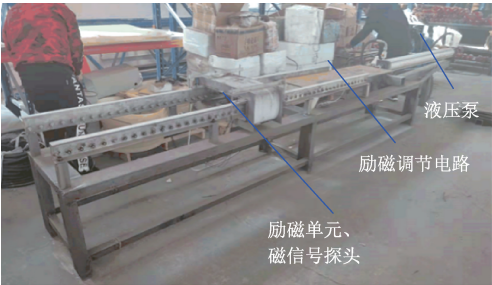
图 15 不同外界磁场缺陷磁信号采集实验设备 Fig. 15 Experimental equipment for magnetic signal acquisition of different external magnetic field defects
