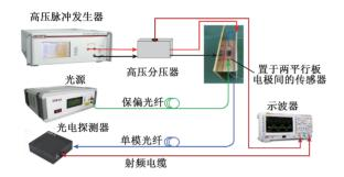
图 4 传感器时域电磁脉冲标定系统 Fig. 4 Calibration system of the sensor in the time
