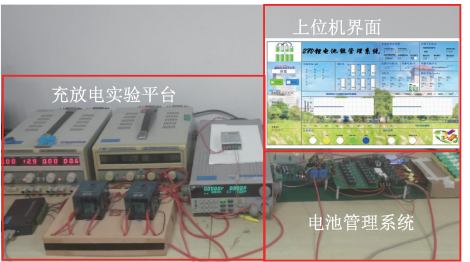
(a) 锂电池充放电测试实验平台 (a) Lithium battery charging and discharging test platform
