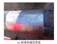
(a) Pipeline with anticorrosive coating
