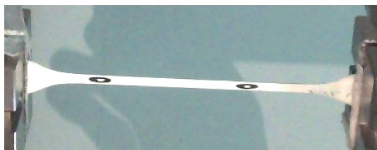
(a) 标记符产生形变 (a) The deformation of marker
