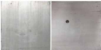
(a) 无缺陷铝板 (a) Aluminum plate with no defects (b) 有缺陷铝板 (b) Aluminum plate with defects
