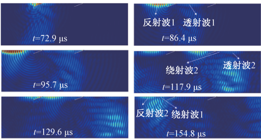
(a) 超声表面波瞬态传播云图 (a) Ultrasonic surface wave propagation process in the rail
