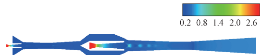
图 12 喷射泵内部流场密度云图 Fig.12 The contour of the flow field density inside the two-stage ejector
