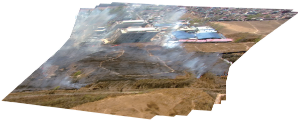
图 17 火灾场景下无人机多路实时视频拼接结果 Fig. 17 Multi-channel real-time video splicing results of UAV in fire scene
