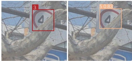
(b) 交通标志误检 (b) False detection of traffic signs
