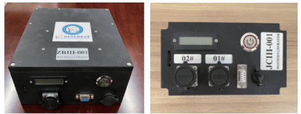
(a) 地电流移动注入终端 (b) 地电场微信号检测设备 (a) Ground current mobile injection terminal (b) Ground current field micro-signal detection
